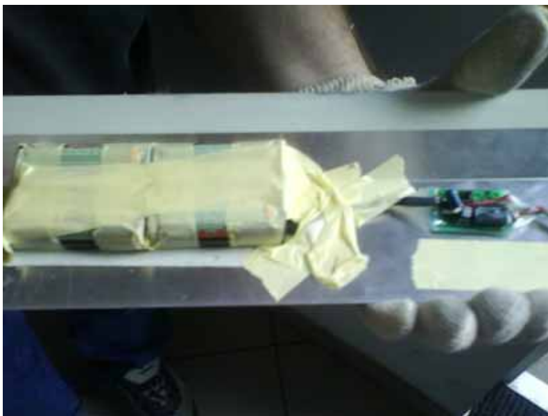
Photo 6 Battery attached to GPRS Phone
