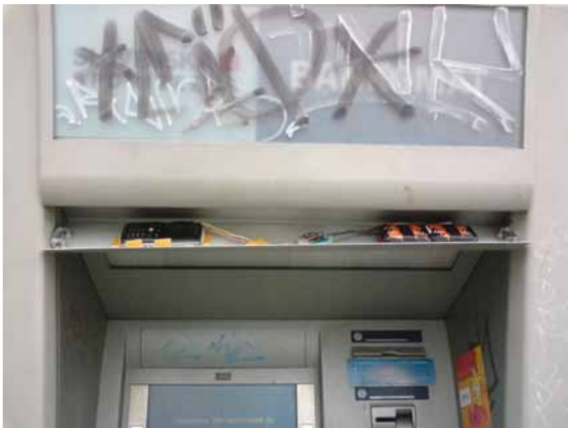
Photo 12 Battery attached to GPRS phone
