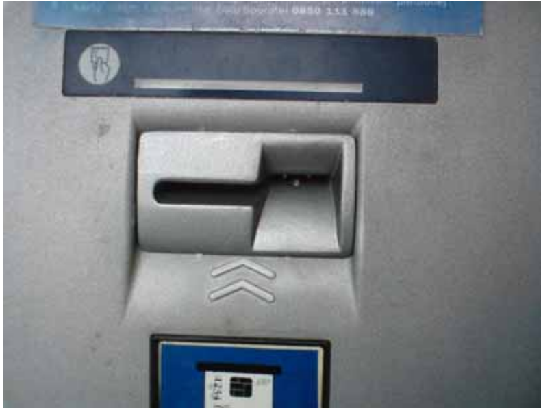
Photo 5 Wincor ATM skimmer inserted
