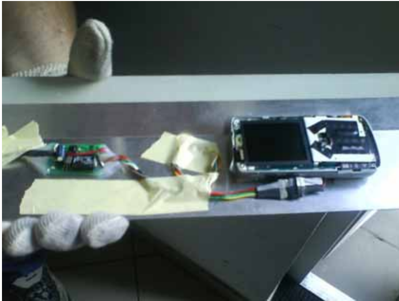
Photo 7 Battery connected to GPRS phone
