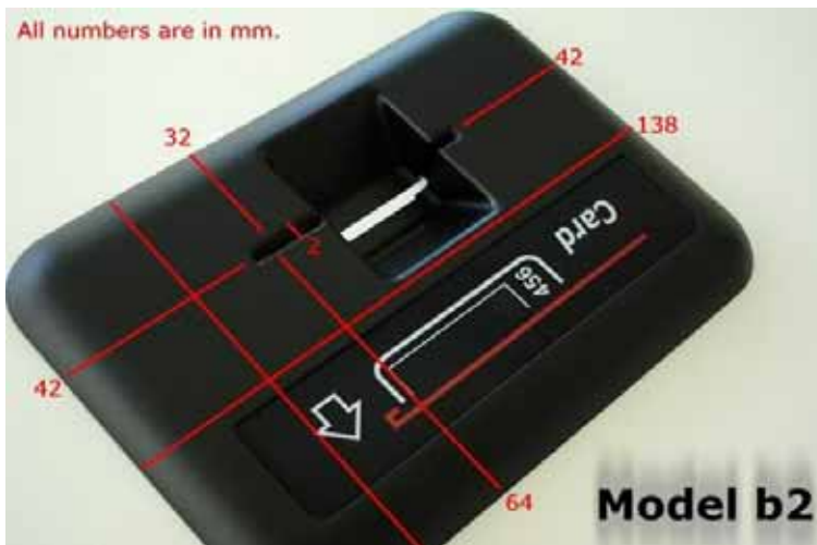
Photo 2 Plastic bezel with invisible skimmer
