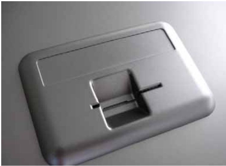
Photo 1 Plastic bezel with invisible skimmer
