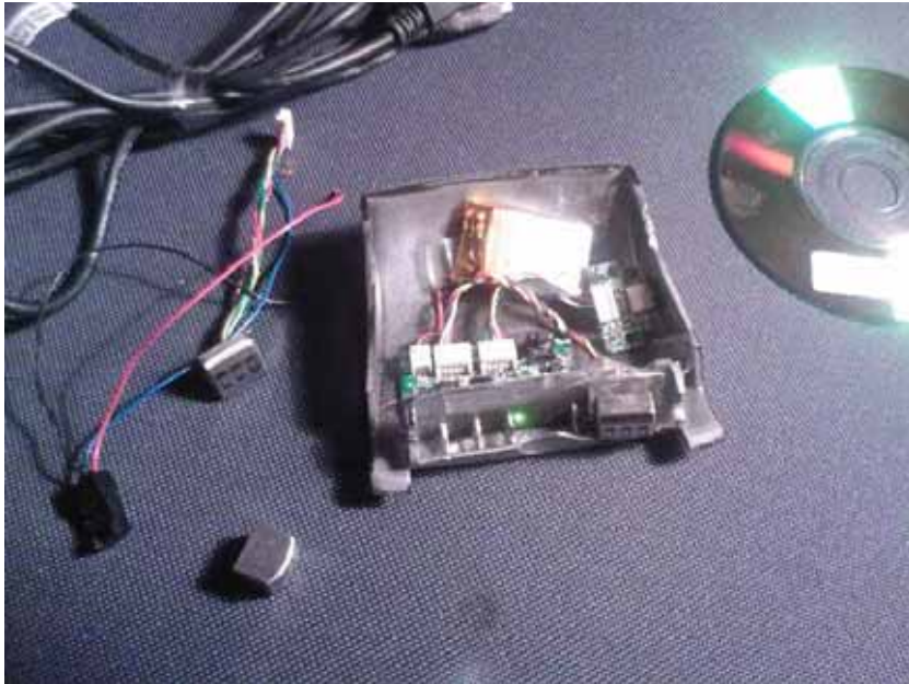
Photo 13 Skimmer hardware inside
