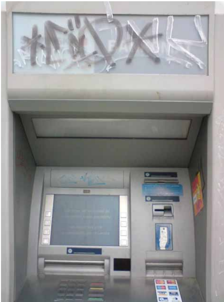
Photo 8 Complete skimset placed on wincor ATM
